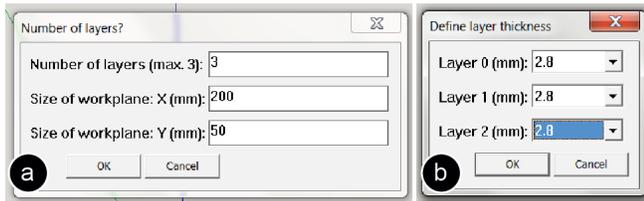
Figure 8: Define (a) number of layers, (b) layer thicknesses.
