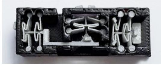
Figure 25: We cross signals by running a crossbar across another cell.
